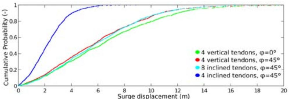
Figure 1: Cumulative probability of full scale surge displacement.
