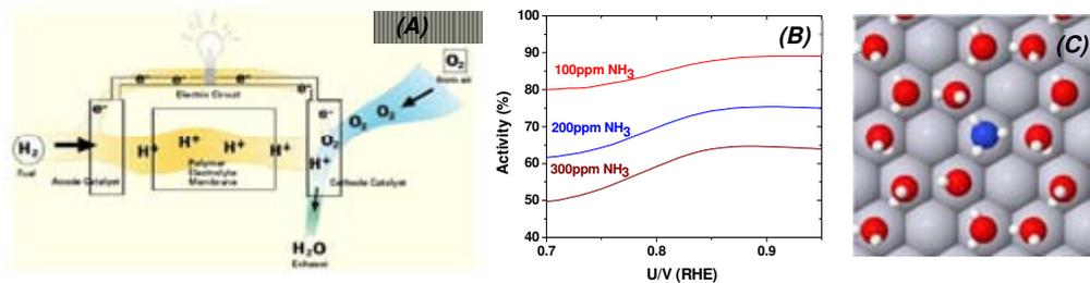
(A) Schematic representation of an operating polymer electrolyte membrane fuel cell. (B) Platinum catalyst ORR activity decrease against applied potential for different ammonia concentrations. (C) Model of an ammonia molecule sitting on top of a platinum catalyst used in the theoretical calculations.
