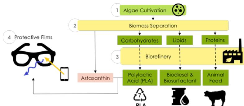
Figure 1: Eyeglass Film Production Method
