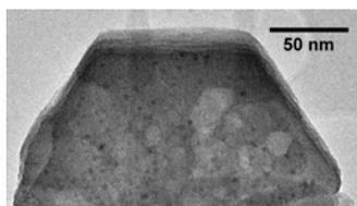
Figure 2: TEM image of metal nanoparticles encapsulated in recrystallized zeolite ZSM-5.
