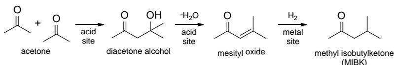
Figure 1: One-step process for production of MIBK from acetone.
