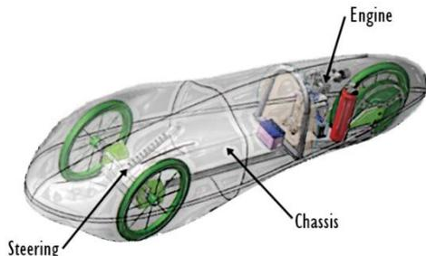
Augmenting engine efficiency involved the sealing of air leaks in the manifold and insulation to assist with the internal combustion reaction. The engine is also retrofitted with a custom fuel injection system that mitigates fuel waste on intake walls by injecting directly at the intake valve for immediate vaporization.
