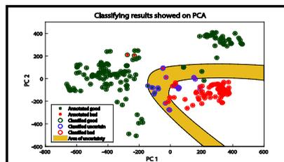
**Figure 1:** The classification model applied on a simulated data set. Notice that this is a projection from 3D to 2D, which results in some of the blue points not being in the yellow region as they should. We get an error rate in the classification of 0.8
