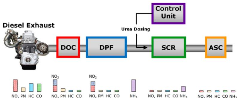
Figure 1: An example of the standard diesel exhaust aftertreatment system<sup>1</sup>.
