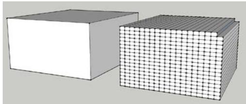
**Figure 1:** Illustration of magnet segmentation
