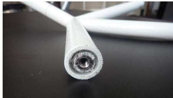
**Figure 5.** 3D-Printed Node with Magnetic Female Connector Part Glued Inside
