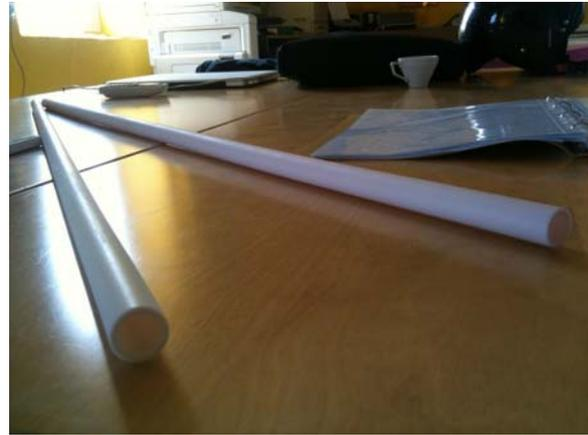
Figure 3. Ceramic Tube Before Enamelling
