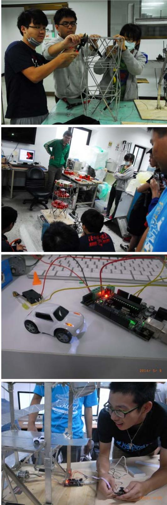
**Figure 2.** Spring 2014 cornersone project: earthquake-resistant automated parking tower. Top: tower assembly and load testing using a shaking table. Bottom: Arduino-controlled model cars and their test drive up and down the tower.
