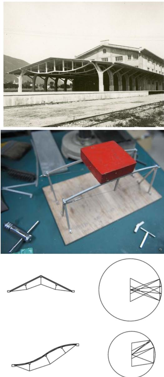
**Figure 5.** Constant chord force trusses and their graphic statics analysis. Top: Robert Maillart's Chiasso Shed (Source: ETH Bildarchiv). Middle: a demonstration structure using jet-cut aluminum and steel cable. Bottom: form and force diagram analysis.
