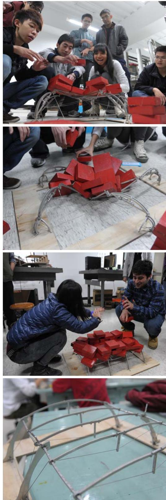
**Figure 7.** Load testing of the roof structures, Spring 2013. Top: students decide to add one more steel block, leading to collapse. Bottom: students argue whether to continue adding weights. They stopped before the structure suffered more than local damage.
