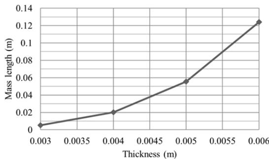
Figure 18. Mass Length as a Function of the Bender Thickness
