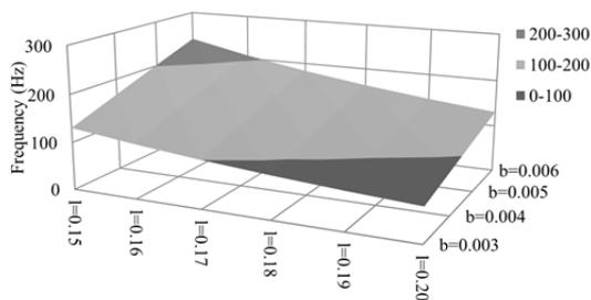
**Figure 12.** Natural Frequency as a Function of the Length and the Thickness for the Aluminum Model
