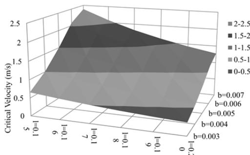
**Figure 15.** Critical Velocity as a Function of the Length and the Thickness for the Lead Model
