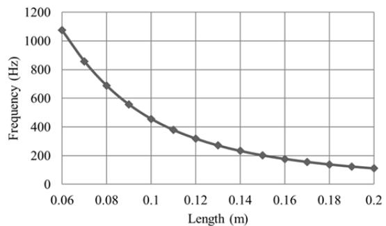
**Figure 4.** Frequency as a Function of the Length
