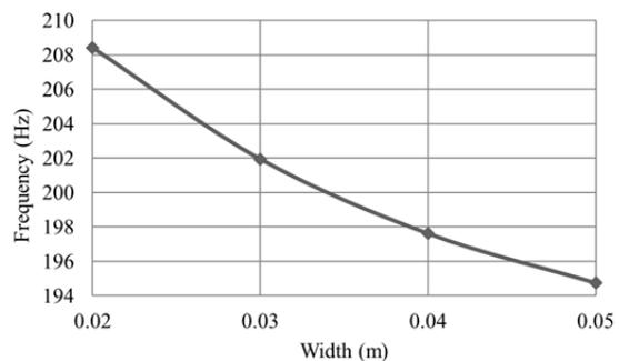
**Figure 5.** Frequency as a Function of the Width
