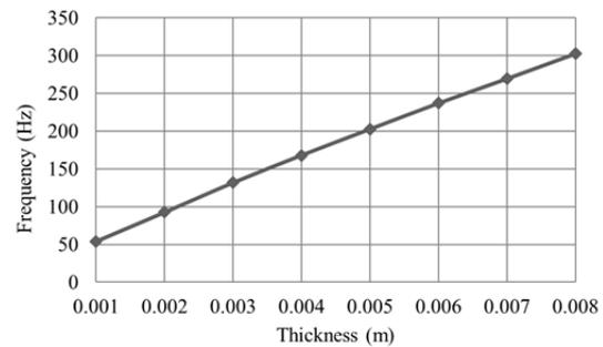
**Figure 3.** Frequency as a Function of the Thickness
