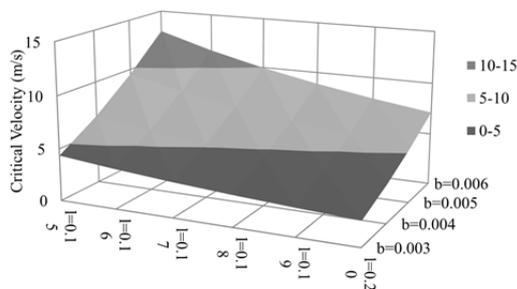
**Figure 14.** Critical Velocity as a Function of the Length and the Thickness for the Aluminium Model
