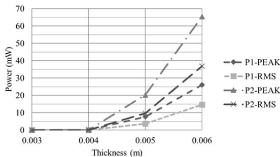
Figure 23. Peak Values and RMS Values of the Power for Different Bender Thicknesses
