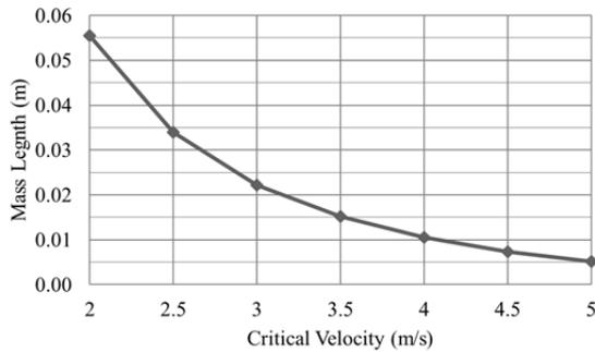
Figure 16. Required Mass Length for Different Critical Velocities
