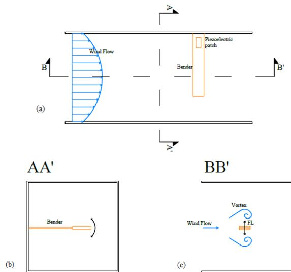
Figure 1. Piezoelectric Bender Inside the HVAC Duct
