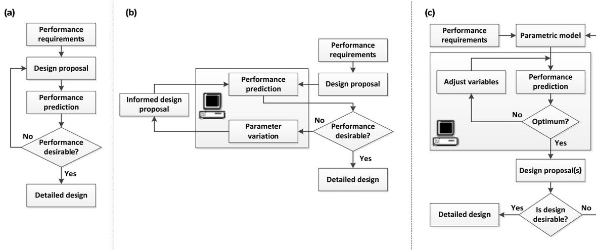
**Figure 2.** Development of the Performance-Based Design Paradigm, (a) Performance-Based Design (Kalay, 1999), (b) Implementation of Parameter Variation to Inform Design Decisions in Performance-Based Design (Petersen, 2010), (c) The Proposed Method that Automates the Generation of Design Proposals.
