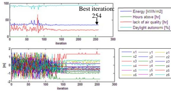
**Figure 8.** Optimisation of North-Oriented Room. Top: Performance. Bottom: The Relative Location of the Variables
