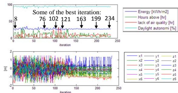
**Figure 10.** Optimisation of South-Oriented Room. Top: Performance. Bottom: The Relative Location of the Variables
