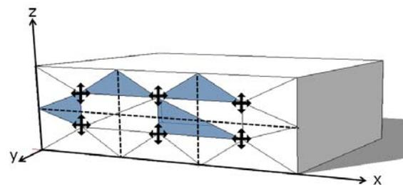
**Figure 7.** Case Example Featuring a Façade Design with Six Variable Nodes in the Façade.
