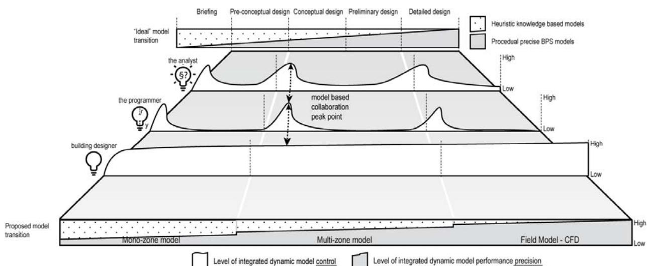
**Figure 3.** Consequence Based Design Framework. Integrated dynamic models are used throughout the design process and benefit from procedural precise calculation models, as described by Shaviv *et al.* (1992), here illustrated with three different types of runtime linked BPS tools. When transitioning from one BPS tool to another, model control collaboration between the operators is required. These can be seen as model based collaboration points.
