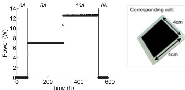
Figure 2: Power of a pre-mixed biogas (60%  $\text{CH}_4$ , 40%  $\text{CO}_2$ ) fueled SOFC with a current up to 16A at 850°C. Anode gas composition: 50% biogas, 40%  $\text{H}_2\text{O}$  and 10%  $\text{H}_2$ . Cathode gas: Air.
