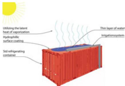
*Cooling container with irrigation system*
