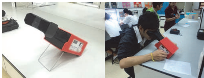
Figure 2: Critical Fusion Frequency test
