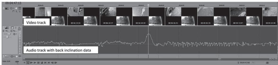
Figure 2. Back inclination data visualized on the audio track in Sony Vegas Pro
