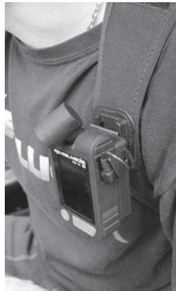
Figure 1. The body worn camera attached with a harness
