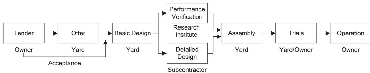
Figure 1. Example of the ship building process. Adapted from (Veenstra & Ludema, 2006)
