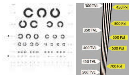
Figure 3: Landolt C optotypes and converging lines on Vidilabs
