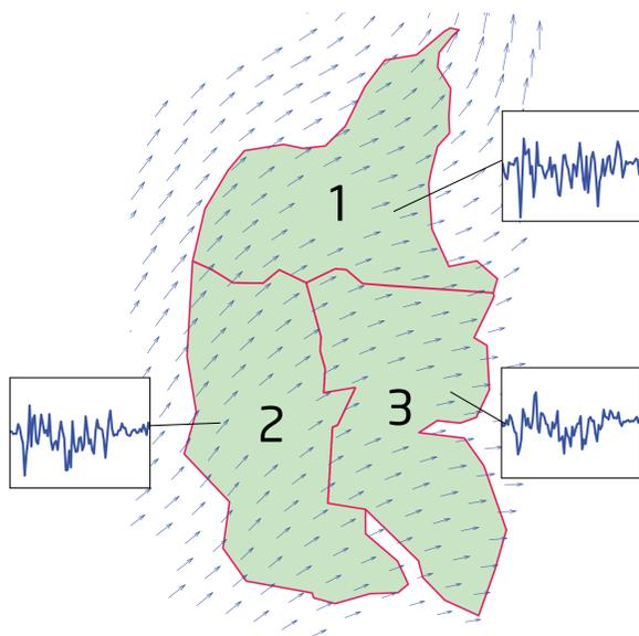
FIGURE 1: Division of the DK1 network into 3 zones. A time series of forecasting errors for each zone is presented together with a snapshot of the wind field at 10m height.
