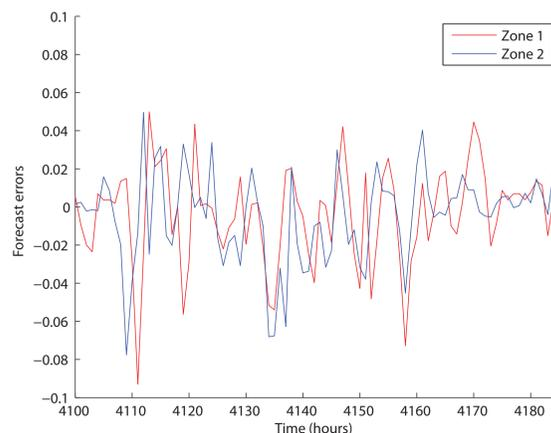
FIGURE 2: Forecasting errors seem to propagate from zone 2 to zone 1.
