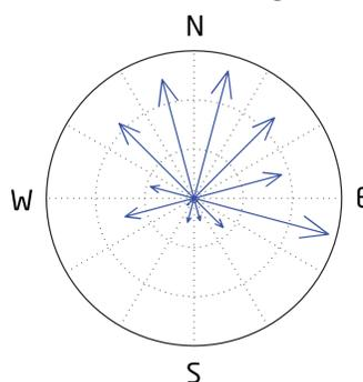
FIGURE 3: Significant wind directions correlating zone 1 and zone 2 with 1 hour delay. For each wind direction, the length of the arrow is the amount of correlation.
