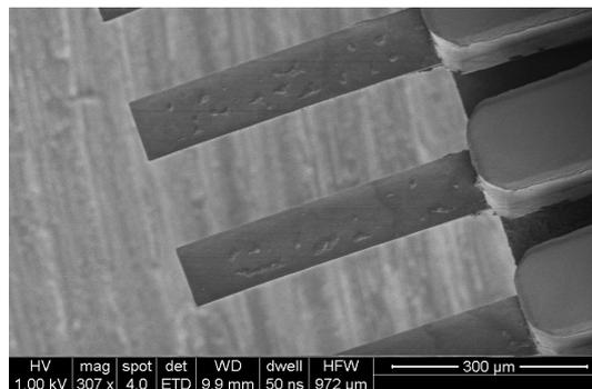
Figure 1: SEM image of PLLA cantilevers after chip release. The support structure is visible to the right.
