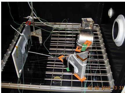
Figure 1 Test setup in free field chamber: 3 objects with TEGs attached. Thin aluminium plate, aluminium triangle and a steel rod.
