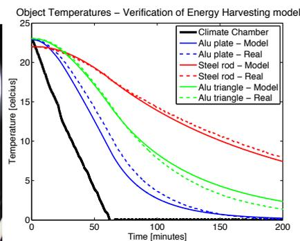
Figure 2 Measured and simulated test object body temperatures. The black line is the surrounding temperature change.
