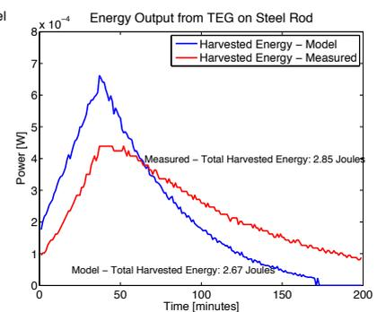
Figure 3 Energy harvested from the steel rod in the free field chamber, measured and simulated.
