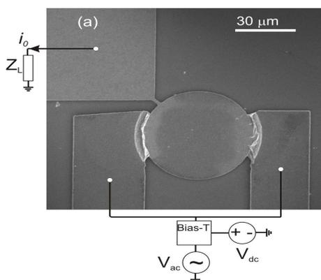
Illustration 1: Figure 1: Picture of the device. Both the disc and the capacitor electrode are seen.
