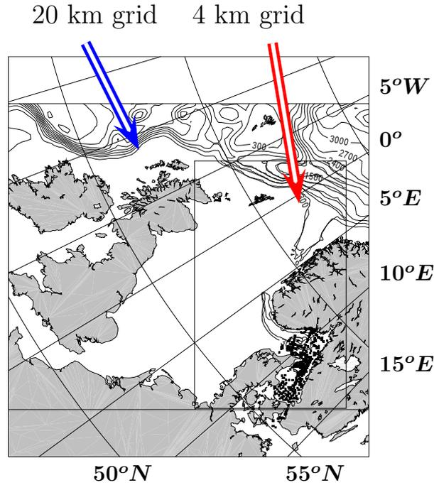
FIGURE 1. Map of the computational domain and the location where validation data are available. Large quadratic area corresponds to the coarse mesh (20 km grid) model, while the smaller rectangular area depicts the fine mesh Skagerrak/northern North Sea area (4 km grid). Heavy black curves indicate bottom topography (300 m contour interval). Locations where validation data for 1998 are available are marked by black dots.
