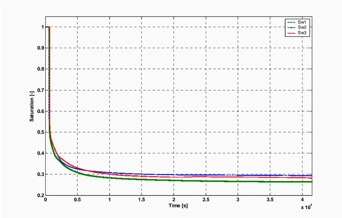
FIGURE 2 . Water saturation versus time at three locations along the sand column.
