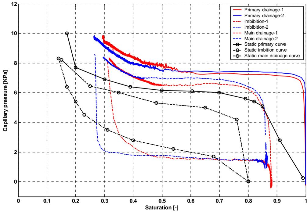
FIGURE 4. Dynamic capillary pressure-saturation curves versus water saturation throughout primary, main drainage and imbibition experiments at applied pressure of 20 kPa.
