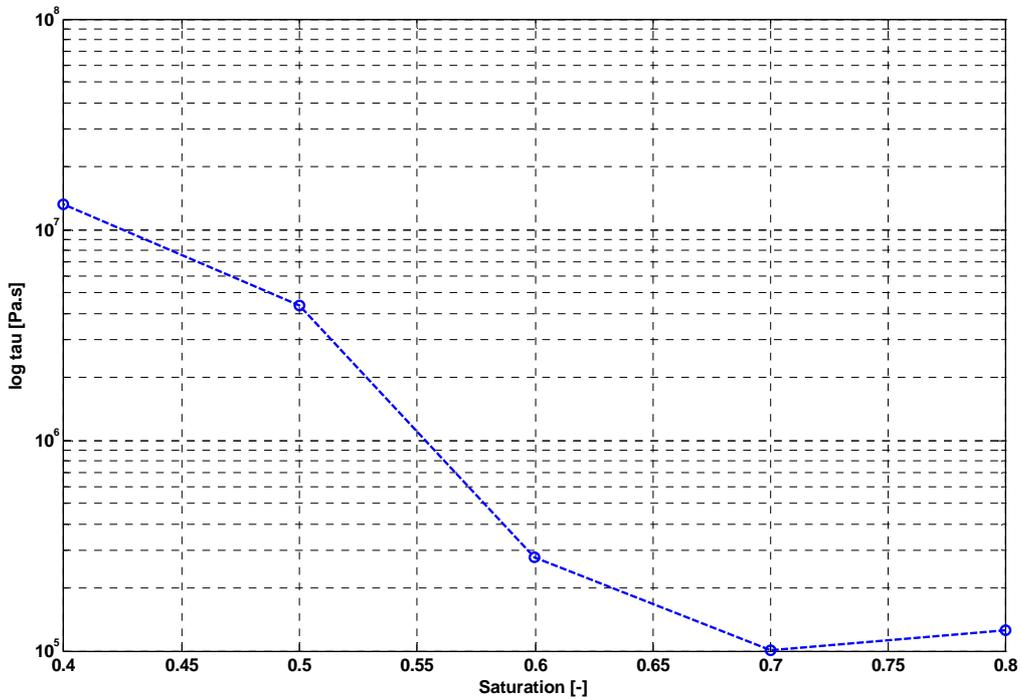
FIGURE 5. Dynamic coefficient  $\tau$  as a function of water saturation.
