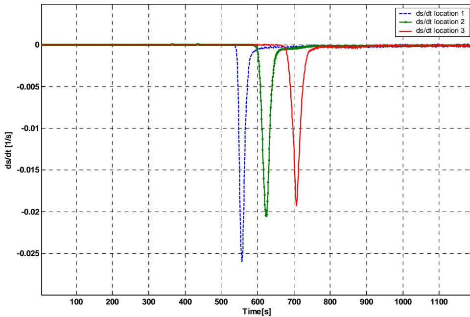
FIGURE 3. Rate of change of water saturation versus time.
