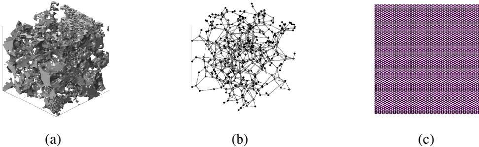
Fig. 1. Berea sandstone sample of size 3mm x 3mm x 3mm from *Øren and Bakke, 2002* (a); A geologically equivalent network (b) and the diamond lattice network (c).
