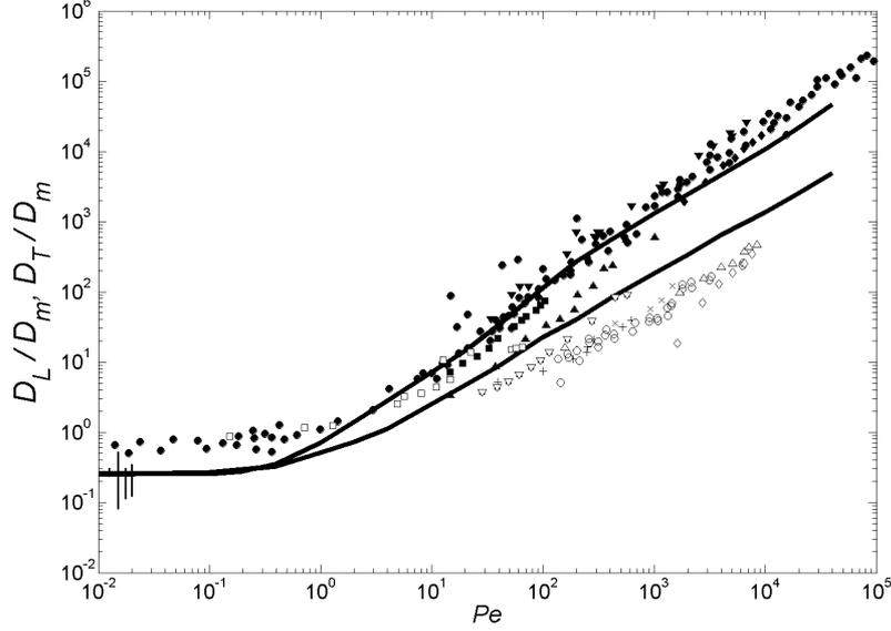
Fig. 2 Comparison of the network model results for longitudinal (upper solid line) and transverse (lower solid line) dispersion coefficients with experimental data (filled symbols for longitudinal dispersion and open symbols for transverse dispersion). The literature sources for the experimental data are given in the text. The sandstone data are presented in the far left side of the figure by the solid lines with error bars.
