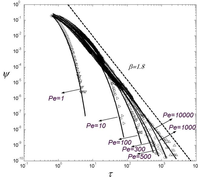
Fig. 3 The probability,  $\psi$ , of traveling between two neighboring pores in a dimensionless time  $\tau = t/t_1$ , where  $t_1$  is the mean travel time  $L/u$ , plotted for different values of  $Pe$  (points). Also shown (lines) are matches using Eq. (1) with a single adjustable parameter  $\beta = 1.8$ . For  $Pe$ ,  $\tau > 5$  Eq. (1) accurately reproduces  $\psi(\tau, Pe)$ . To illustrate the power-law scaling a dashed line of slope  $1+\beta$  is indicated on the graph.
