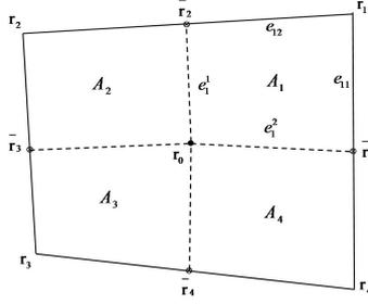
FIGURE 1. A quadrangular cell  $A$  and the four subcells  $A_k$ .
