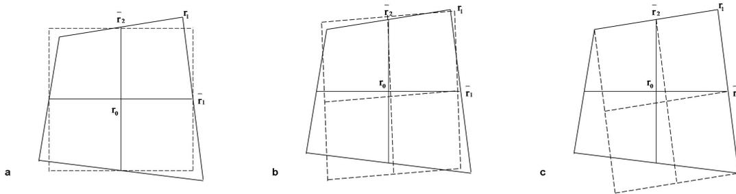
FIGURE 3. The transformation of the quadrilateral subcell  $A_1$  into an approximative parallelogram which is based on midpoint (a), mean integrate (b) and corner-point (c) Jacobian evaluation
