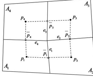
FIGURE 2. An interaction region  $I$  constituting by the four subcell  $A_i$  where  $\bullet$  correspond to the mean pressure evaluation  $p_i$  and  $\otimes$  the mean pressure evaluation  $\bar{p}_i$  on the inner edge of  $I$ .
