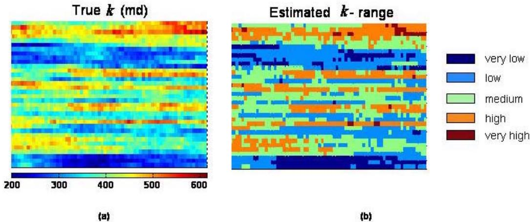
FIGURE 3. (a) True permeability field of the Berea sandstone slab obtained using *AutoScan*. (b) Estimated permeability-range field obtained using the proposed methodology based on belief theory.
