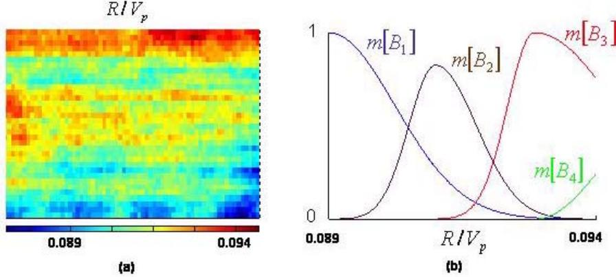
FIGURE 2. (a) Ratio of Resistivity and Velocity data ( $R/V_p$ ). (b) Basic mass assignments. At a given  $R/V_p$ ,  $m[B_i](R/V_p)$  represents the the basic mass of focal  $B_i$ , which is a subset of possible conductivity ranges that the geophysicist thinks  $R/V_p$  implies.
