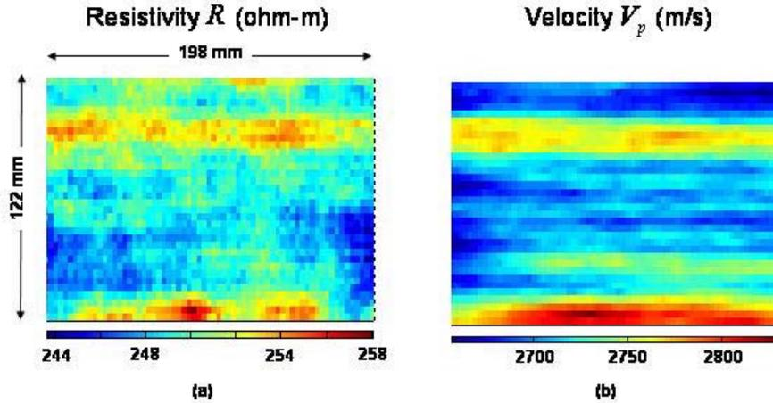
FIGURE 1. *AutoScan* data maps of Berea sandstone used in the study: (a) resistivity. (b) acoustic velocity (shear wave).
