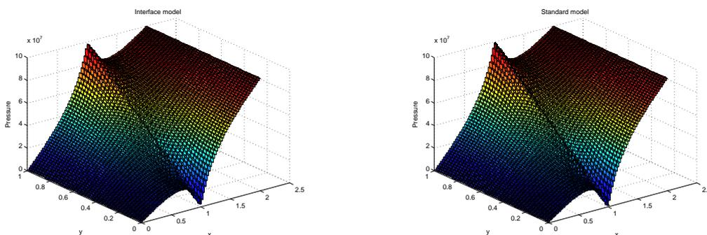
FIGURE 3. Pressure for the interface fracture model (left) and reference pressure (right)
