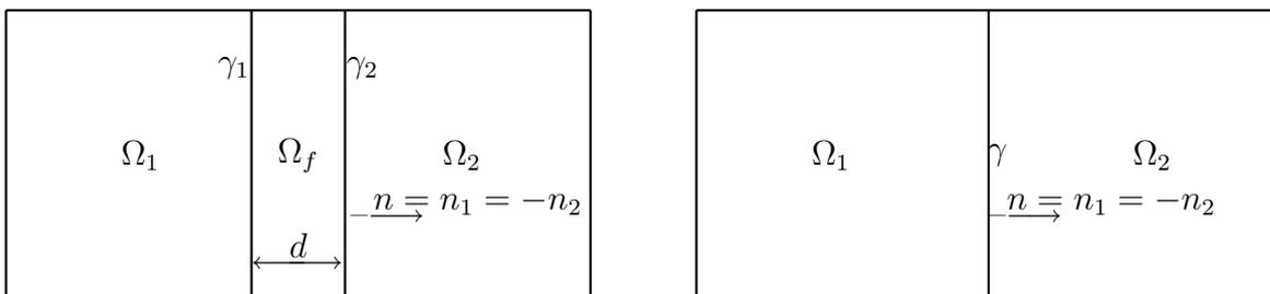
FIGURE 1. Left: the domain  $\Omega$  with the fracture  $\Omega_f$ . Right: the subdomains  $\Omega_1$  and  $\Omega_2$  separated by the fracture considered as an interface  $\gamma$ .
