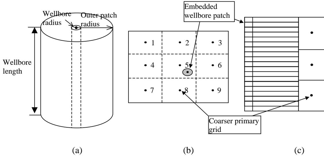
FIGURE 1. A schematic of the wellbore patch and the patch embedded in a coarser primary grid. Figure 1a shows details of the wellbore patch, 1b shows the embedded wellbore patch in a planar view, 1c shows the embedded wellbore patch in a vertical view.
