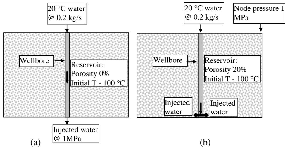
FIGURE 2. A schematic diagram showing the configuration of the comparison problems. Figure 2a shows configuration for heat transfer only problem where water flows only through the wellbore. Figure 2b shows the configuration for heat and mass transfer problem where water flows through the wellbore and in the reservoir through the bottom node.
