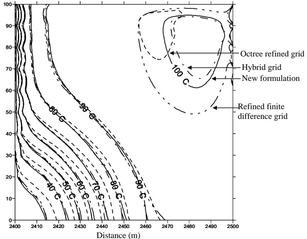
FIGURE 4. Comparison of temperature profiles near the wellbore (at 2400 m) along a vertical plane. Solid lines show contours for new formulation, dash-dot lines show contours for hybrid grid, uniform dashed lines show contours for octree refined grid and mixed dashed lines show contours for refined finite difference grid.
