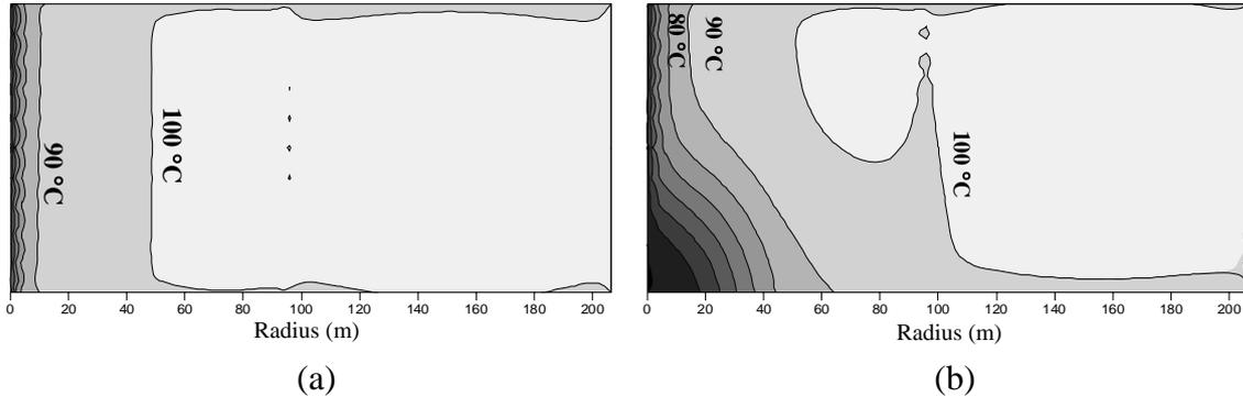
FIGURE 3. Comparison of temperature profiles along the radial direction. The wellbore is at 0 m. The solid lines show the contours for embedded wellbore patch. The filled contours show the contours for radial grid used for comparison. Figure 3a shows results for heat transfer only problem. Figure 3b shows results for heat and mass transfer problem.
