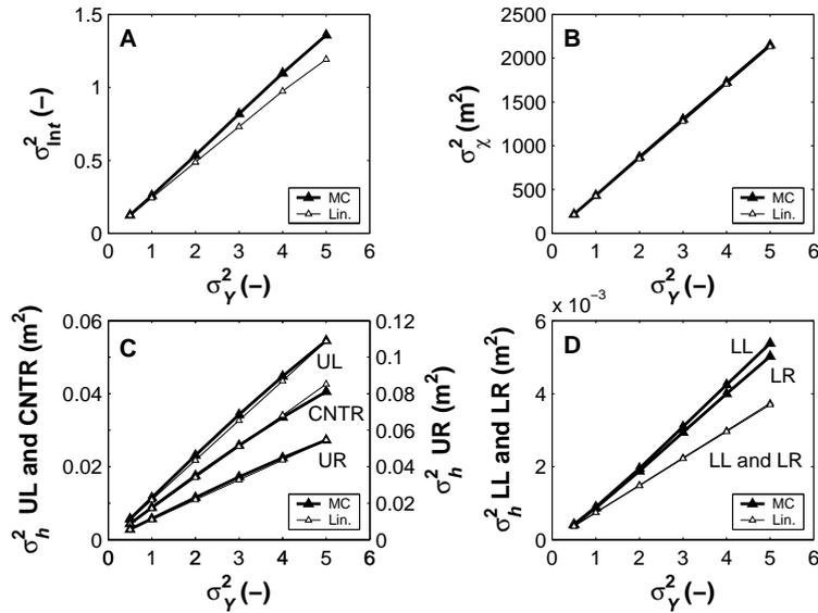
FIGURE 2. Comparison of linearized  $t$  (a),  $\chi$  (b) and  $h$  (c and d) variance predictions as given by the representer approach with variances obtained from a Monte Carlo series, as function of  $\sigma_Y^2$ . In (c and d), the labels UL, LL, UR, LR and CNTR correspond with the labels in Figure 1 and indicate the locations in the domain at which the variances were evaluated.
