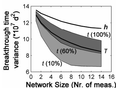
FIGURE 3. Breakthrough time uncertainty reduction achieved by networks consisting of only one observation type, as a function of network size. The percentages given refer to different levels of the age observation error standard deviation.
