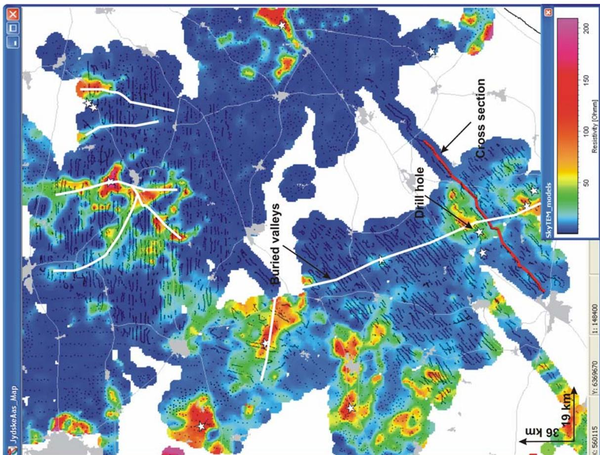
Figure 4. The map shows the average resistivity in the interval from 60 - 40 m below sea surface. The major valleys are filled with high resistive sediments - probably sand and gravel.
