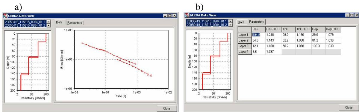
Figure 6. The figure shows an example of a dataset at position 8500 m in Figure 5. The two curves in a) shows the low moment and the high moment data. The plot to the left shows the inverted model which are also shown in b). b) shows the estimated model parameters which are resistivities, thicknesses and depths and their uncertainty (standard deviation, STD) expressed as factors.
