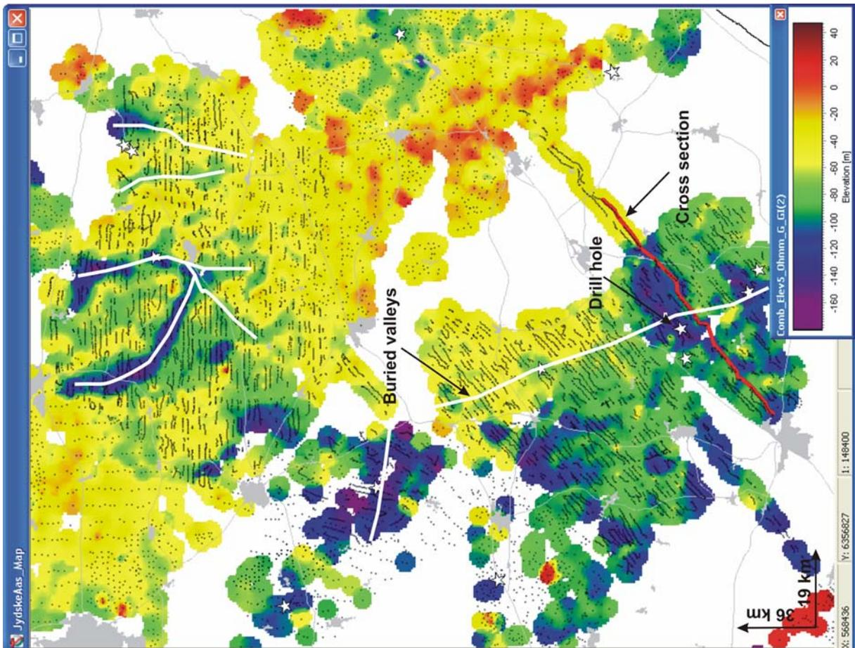
Figure 3. The map shows the elevation of the low resistivity layer. The black dots are the transient sounding points, gray lines show the major roads and houses and the white lines outline some of the major buried valleys. The white stars show the location of the investigation drillings. The red line show the location of the section in Figure 5
