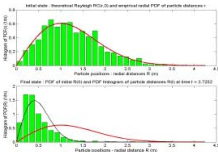
FIGURE 3. Radial particle plot, and fitted Rayleigh distribution,  $C(r)$ , during 2D anti-diffusion starting from Gaussian plume on top.
