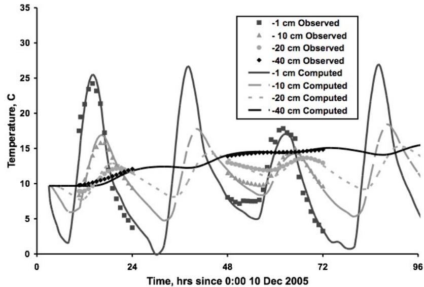
FIGURE 4. Comparison of predicted and observed physical temperatures at different depths below ground surface at the desert site.
