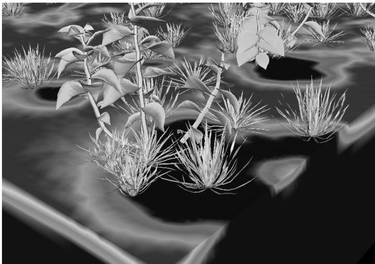
FIGURE 5. Temperature contours on the vegetation and the soil. The darkest regions are cool areas caused by the plant shadows. The scene has about 4 degree C range in temperature.
