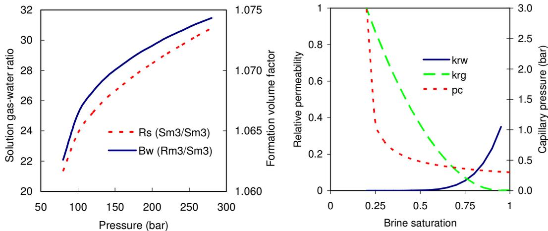
FIGURE 2: Black oil properties (a) and saturation functions (b) used in calculation examples.
