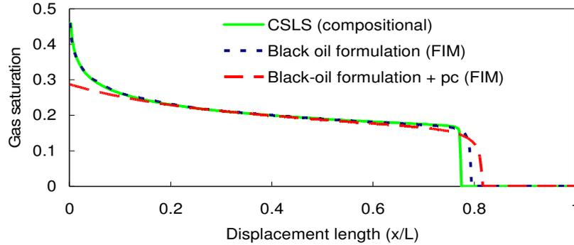
FIGURE 3: 1D displacement calculations using CSLS and FIM: Impact of capillarity.
