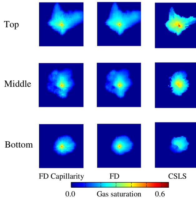
FIGURE 6: Effects of capillarity on CO<sub>2</sub> plume
