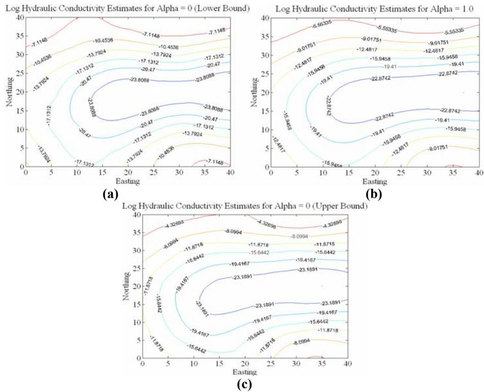
FIGURE 5 (a) – (c): Contour plots of updated fuzzy estimates for (a) lower bound of the zero  $\alpha$ -cut, (b) the median values ( $\alpha = 1$ ), (c) upper bound of the zero  $\alpha$ -cut.
