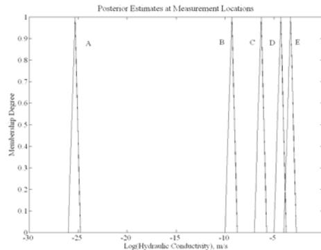
FIGURE 6: Posterior estimates at all measurement locations; Measured values are: -25(A), -9(B), -6(C), -4(D), -3(E)
