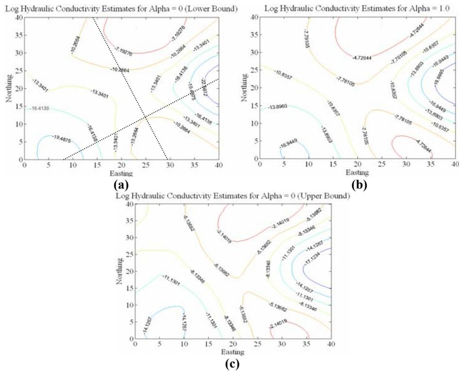
FIGURE 4 (a) – (c): Contour plots of kriged fuzzy estimates of log hydraulic conductivity for (a) lower bound of the zero  $\alpha$ -cut, (b) the median values ( $\alpha = 1$ ), (c) upper bound of the zero  $\alpha$ -cut.
