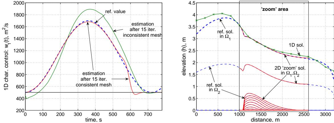
FIGURE 4. Reference boundary condition and its estimations for consistent/inconsistent mesh (left); reference flow and the 1D/2D 'zoom' solutions by JAC for inconsistent mesh (right)
