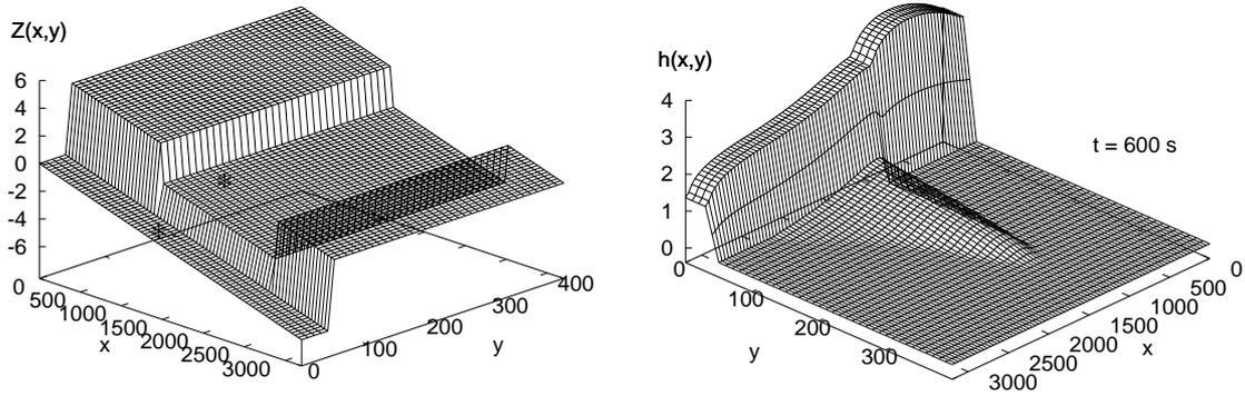
FIGURE 2. Bathymetry(left) and reference flow (right)
