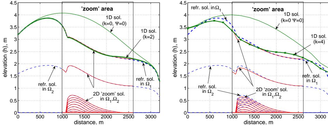
FIGURE 3. Reference flow and the 1D/2D 'zoom' solutions by WFR method for consistent (left) and inconsistent mesh (right)
