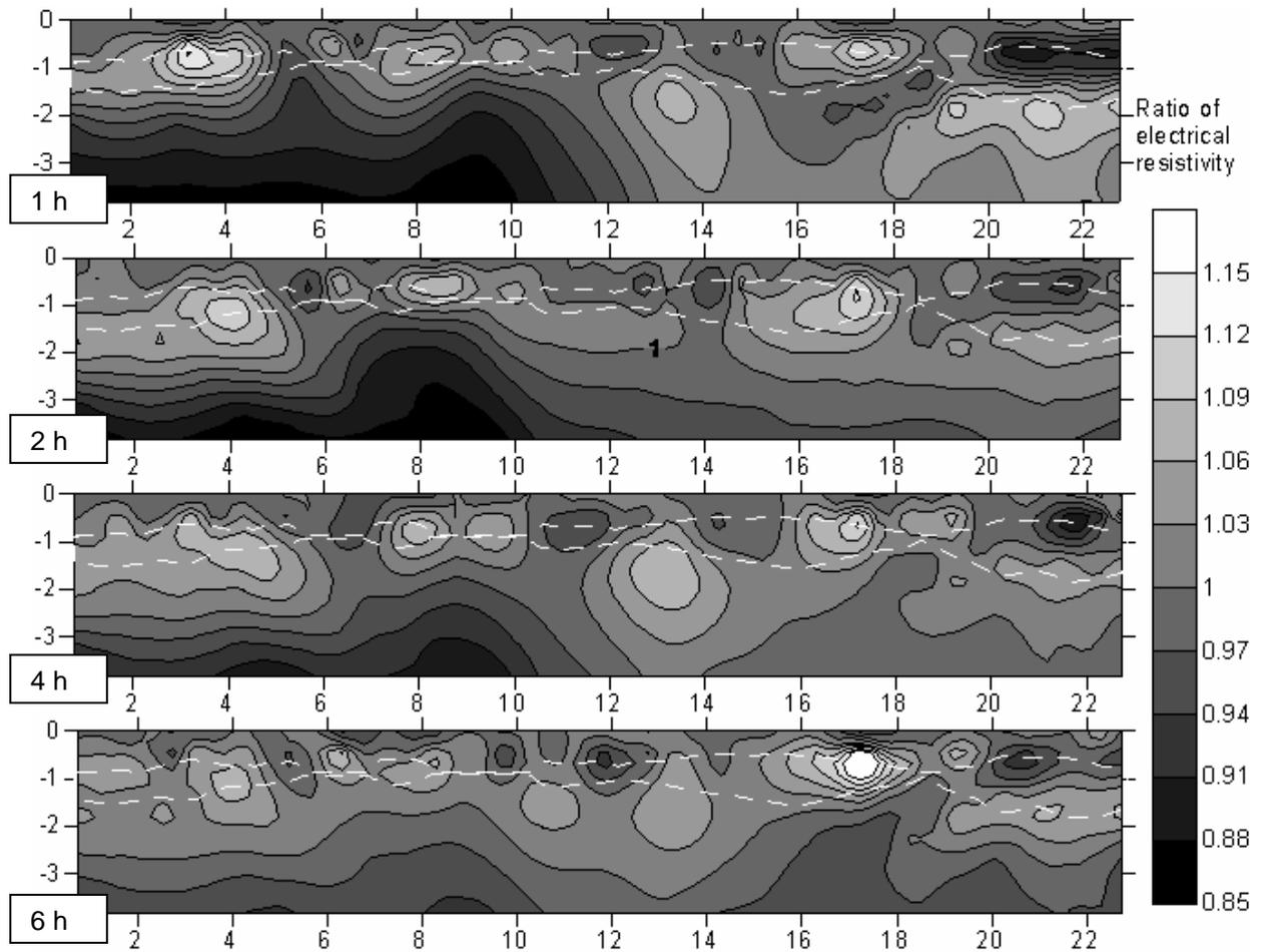
FIGURE 4. Values of electrical resistivities normalised on measurements conducted directly after injection in pipes. Numbers of hours from pulse injection indicated. White stippled lines indicate coarse layer interpreted from Fig. 3
