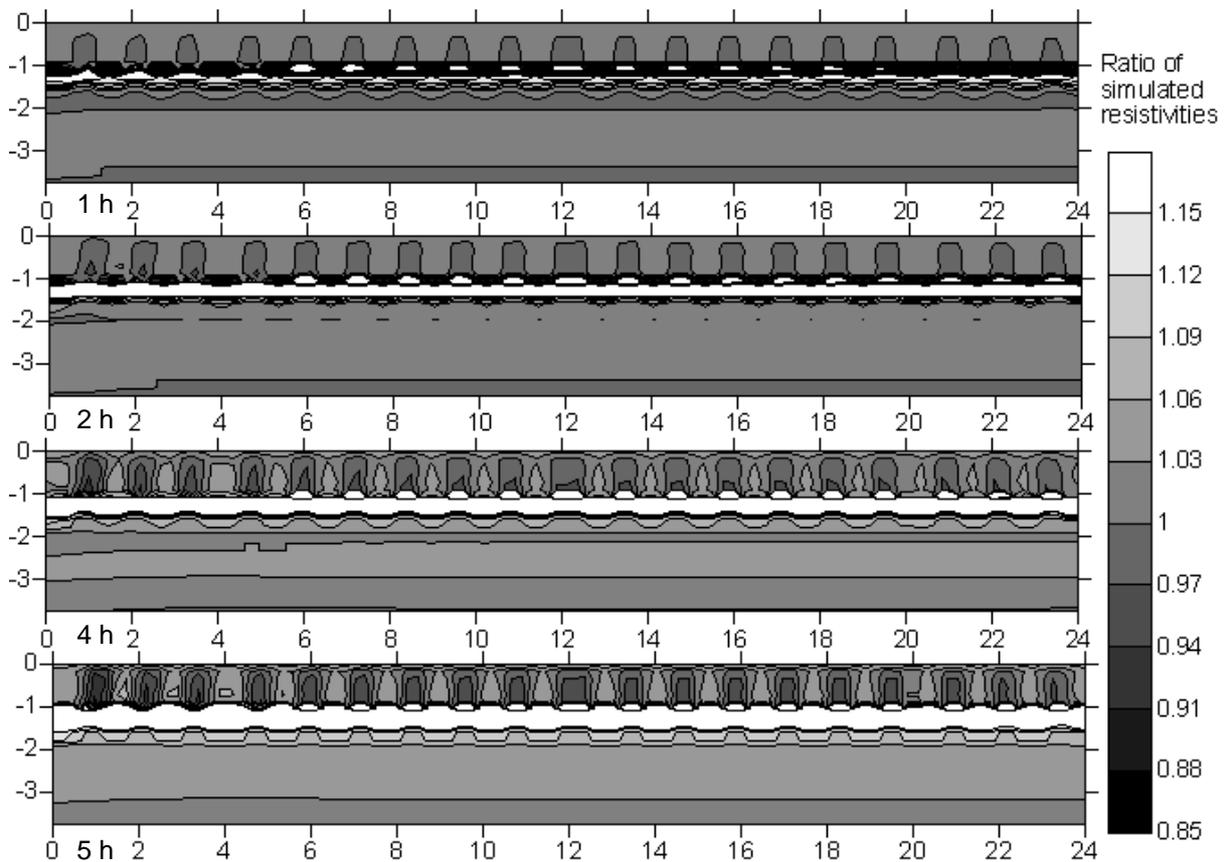
FIGURE 2. Values of ratio resistivities estimated from numerical simulations. Normalised on modelling results of 0.5 hours pipe injection. Time (hours) from pulse injection indicated.
