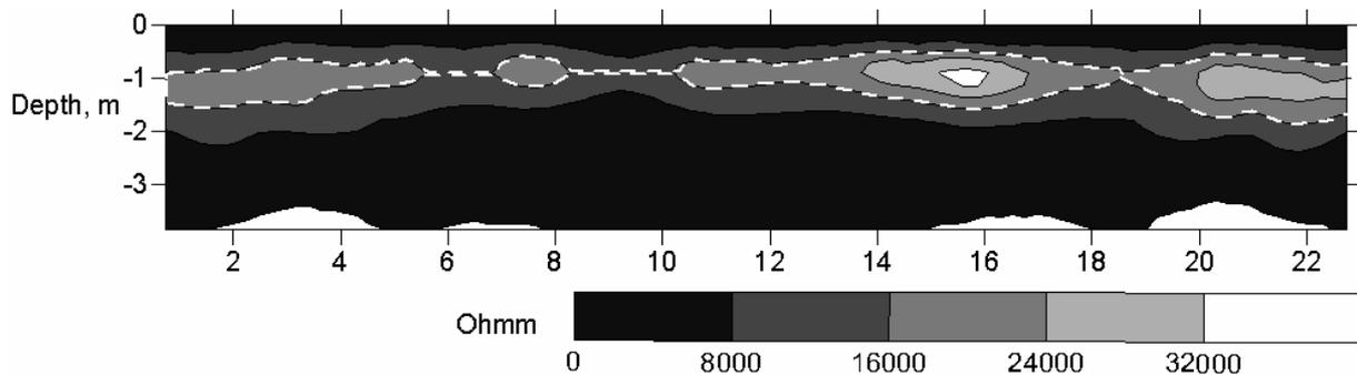
FIGURE 3. Electrical resistivities measured along a 24 m long line perpendicular to distribution pipes. White stippled lines indicate what is interpreted as the distribution layer.
