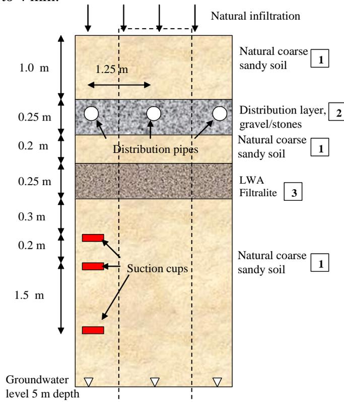
FIGURE 1. Vertical section through part of the infiltration system, with layers of different soil properties (bold), stippled part was used for verification of numerical model.
