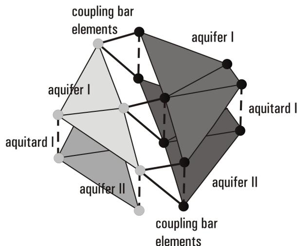
FIGURE 2. Meshes of two models coupled by finite bar elements.
