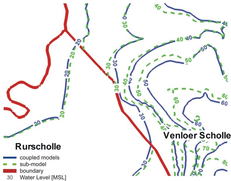
FIGURE 3. Isolines of the top aquifer water level: simulation results of the coupled model and the sub-models
