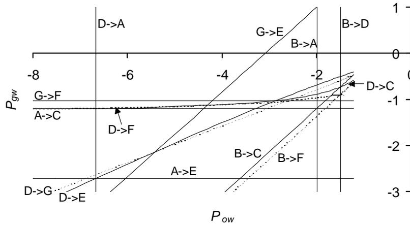
FIGURE 4. Capillary entry pressures and layer displacement criteria in terms of  $P_{gw}$  versus  $P_{ow}$  for the water flood displacements (vertical lines) and the displacements during the subsequent gas invasion.
