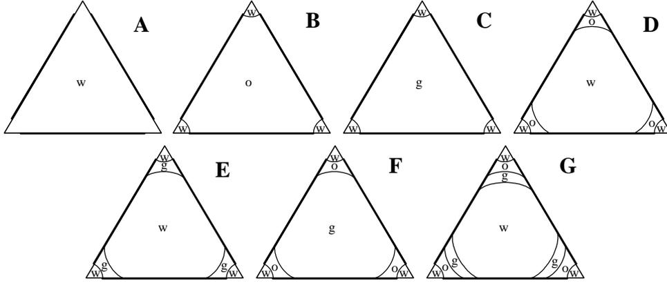
FIGURE 2. Cross-sectional configurations associated with three-phase gas invasion, when gas is wetting to water on the surface of altered wettability.
