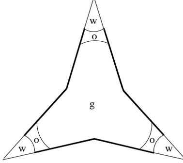
FIGURE 1. Cross-section of a star-shaped pore with water wetting layers in the corners, gas in the centre and oil layers in between. Bold lines indicate surfaces of altered wettability.
