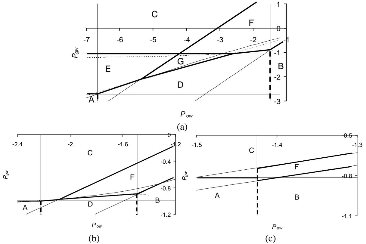
FIGURE 5. Delineation of the  $(P_{ow}, P_{gw})$  space with respect to the various configurations as presented in Figure 2 using the bold lines for the relevant parts of the displacement criteria for (a)  $P_{ow}^{MSP} / P_{ow}^{dr} = 0.1$ , (b)  $P_{ow}^{MSP} / P_{ow}^{dr} = 0.3$  and (c)  $P_{ow}^{MSP} / P_{ow}^{dr} = 0.5$ .
