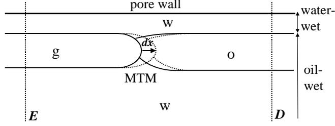
FIGURE 3. Slice along the pore through one of the corners for a small movement  $dx$  of the main terminal meniscus (MTM) associated with displacement  $D \rightarrow E$ .
