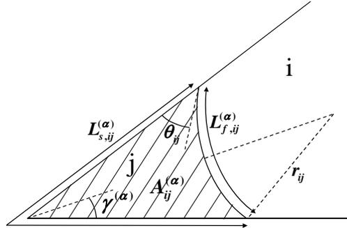
FIGURE A.1 Cross-sectional area  $A_{ij}^{(\alpha)}$  occupied by phase  $j$  in corner  $\alpha$  in the presence of bulk phase  $i$ , where the lengths of the surrounding fluid-solid and fluid-fluid contact lines are indicated as  $L_{s,ij}^{(\alpha)}$  and  $L_{f,ij}^{(\alpha)}$ , respectively.
