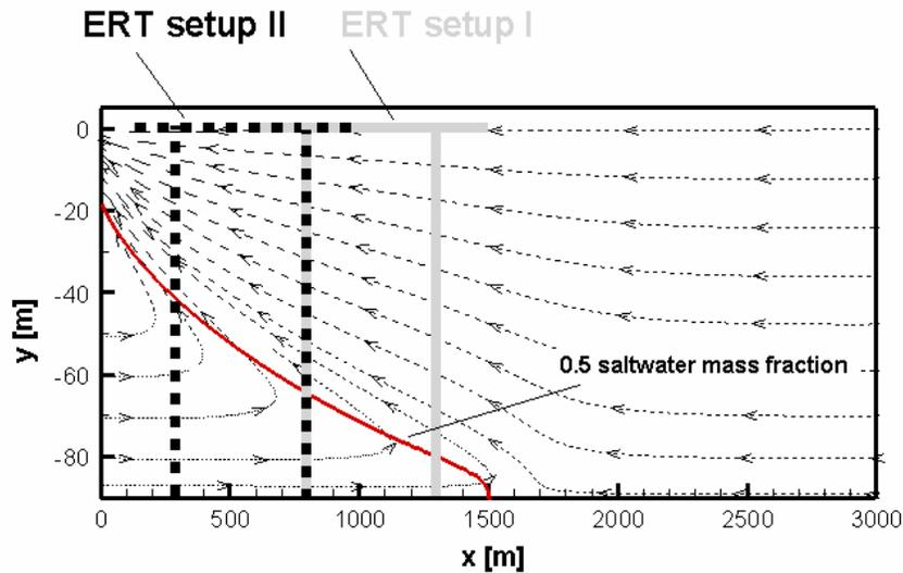
FIGURE 3. Location of surface and borehole electrodes for ERT setup I & II. Location of 0.5 saltwater mass fractions at steady state and associated flow lines.
