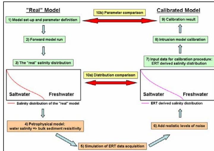
FIGURE 1. A flow diagram illustrating the methodology. Steps 1 – 3 and 7 – 9 (green) involve flow and transport modeling, steps 4 – 6 (orange) ERT acquisition modeling and step 10 (yellow) is results.
