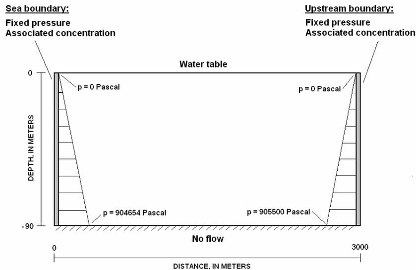
FIGURE 2. Domain geometry and boundary conditions for the synthetic saltwater intrusion model (not to scale).
