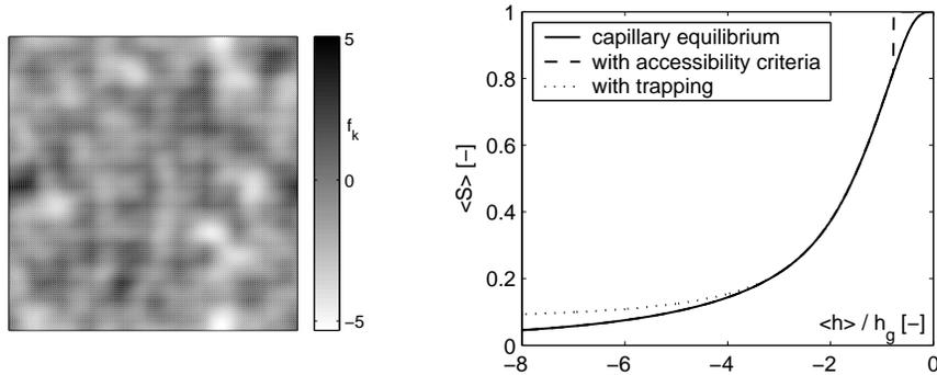
Figure 1: Test field (connected inbetween  $f_k = -0.5$  and  $f_k = 0.5$ ) and effective retention function according to (7), (9) with a ratio of the permeability of 100 as trapping criterion and according to (8).
