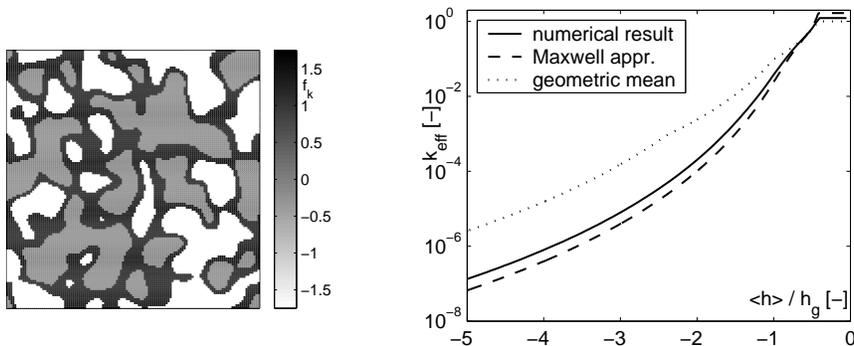
Figure 2: Test field (left) and effective unsaturated permeability curves (right).
