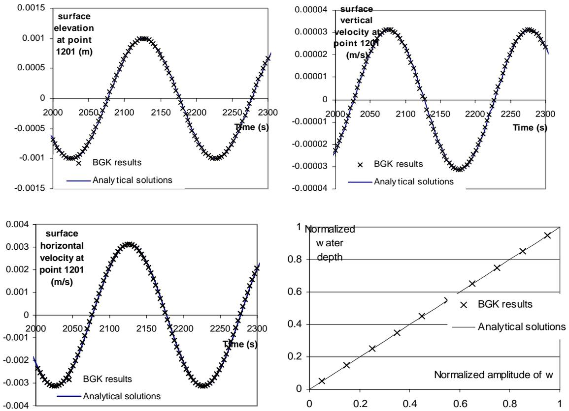
FIGURE. 1 (up left) surface elevation at the water surface at 1200 m from the inflow from 2000 to 2300 s; (up right) surface vertical velocity at the water surface at 1200 m from the inflow from 2000 to 2300 s; (down left) surface horizontal velocity at the water surface at 1200 m from the inflow from 2000 to 2300 s; (down right) Amplitude of vertical velocity.
