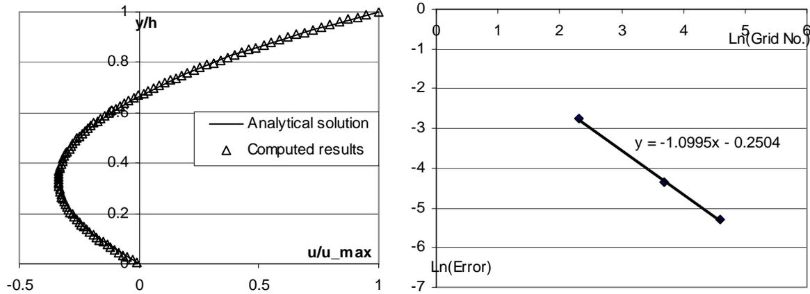
FIGURE. 2. (left) Velocity profile of a wind-driven current with constant eddy viscosity; (right) Convergence study.
