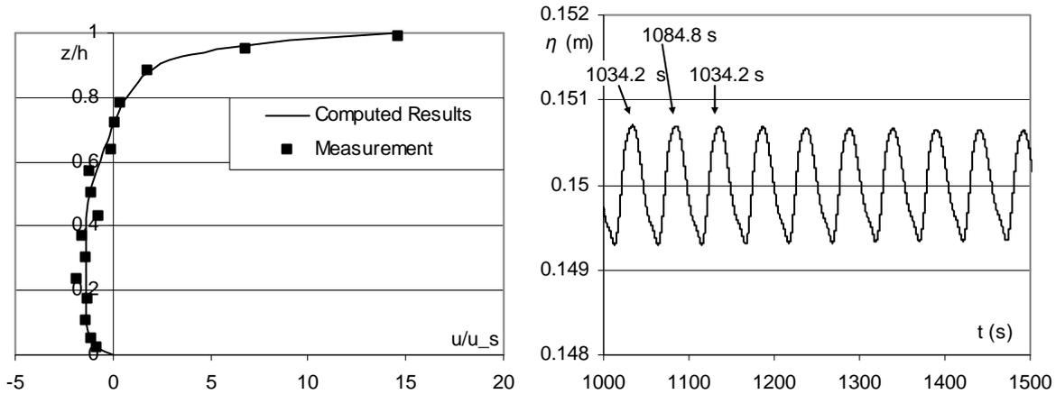
FIGURE. 3 (left) velocity profile of a wind-driven current with parabolic distribution of eddy viscosity; (right) time history of free surface displacement after the initiation of wind
