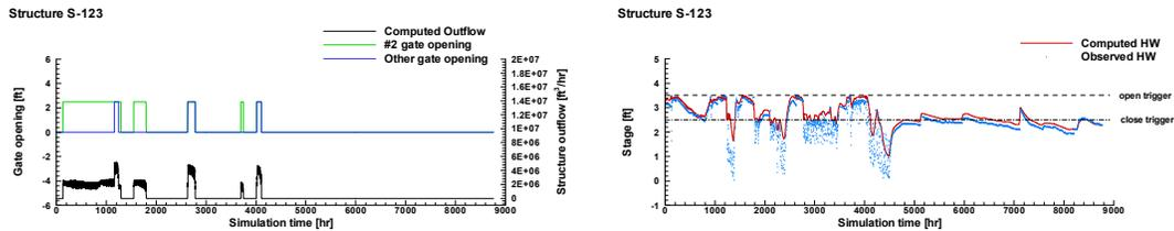
FIGURE 4. WASH123D computational results to verify the implementation of canal structure operation rules.
