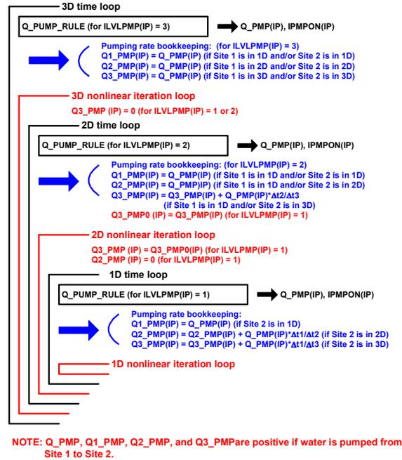
FIGURE 3. Inter-dimensional pumping in WASH123D for a coupled 1D canal network, 2D overland, and 3D subsurface watershed system
