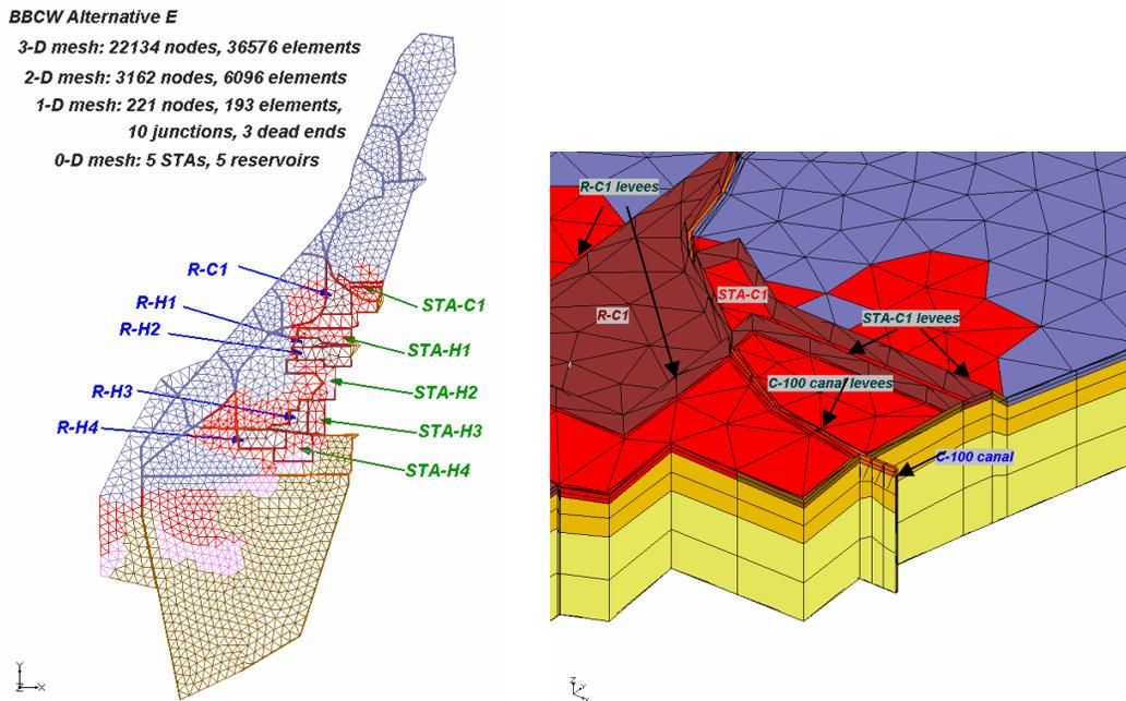
FIGURE 2. WASH123D-BBCW computational mesh for Alternative E: levees are represented with raised elevation to serve as surface water divides (right).
