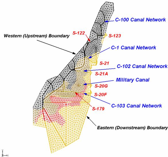
FIGURE 1. WASH123D-BBCW computational mesh for Existing Condition.
