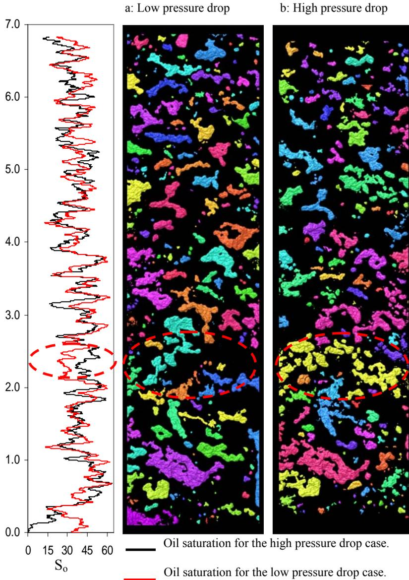
FIGURE 4. Oil distribution low pressure drop (a). Oil distribution high pressure drop (b).
