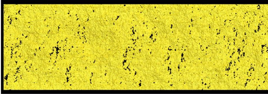
FIGURE 2. A top view of a three-dimensional rendition of the fracture at 3.5 MPa. Black regions are asperities.
