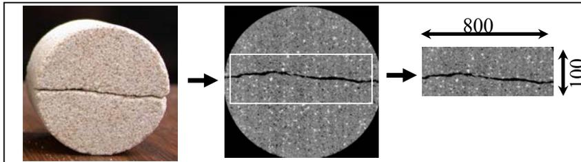
Figure 1: Original core before and after scanning and an extracted region that contains the fracture
