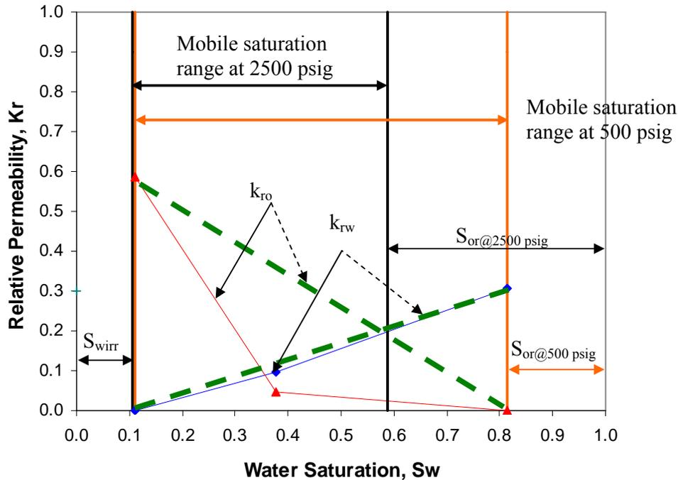
FIGURE 3. Relative permeability curves for a fractured system at 3.7 MPa.
