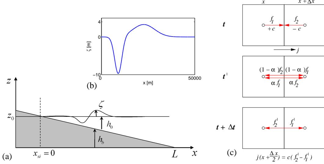
FIGURE 1. (a) Definition sketch of wave run-up study. (b) Initial wave profile. (c)  $D_1Q_3$  model.
