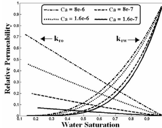
FIGURE 3. Dependency of estimated relative permeability curves with the flow rate
