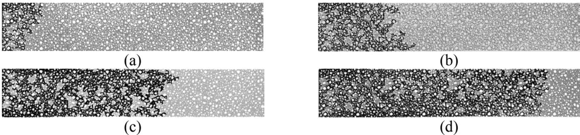
FIGURE 1. Oil saturation evolution during primary drainage process for  $Ca = 1.6 \times 10^{-6}$
