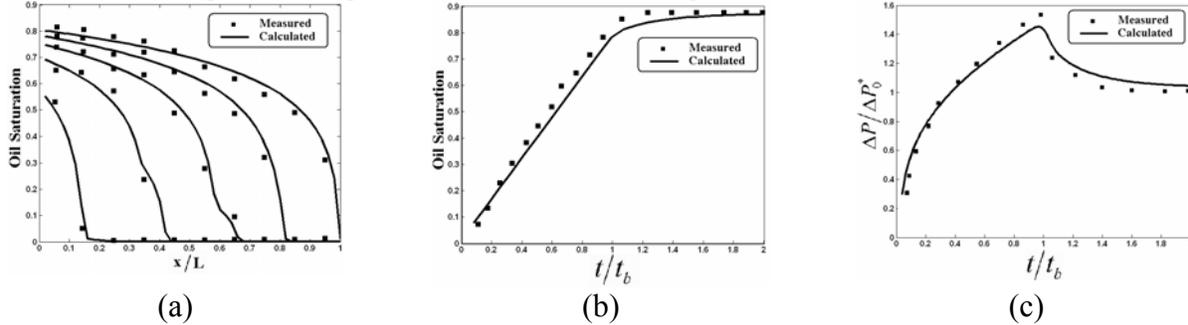
FIGURE 4. Experimentally measured and numerically prediction comparison for  $Ca = 1.6e-6$
