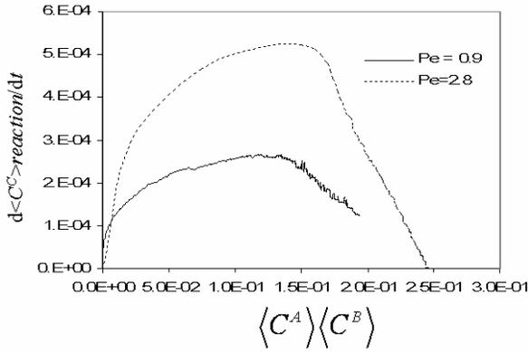
FIGURE 3. Rate of change of  $\langle C^C \rangle$  due to reaction between solutes  $A$  and  $B$  versus the product of the average concentrations  $\langle C^A \rangle \langle C^B \rangle$  for two Peclet numbers.
