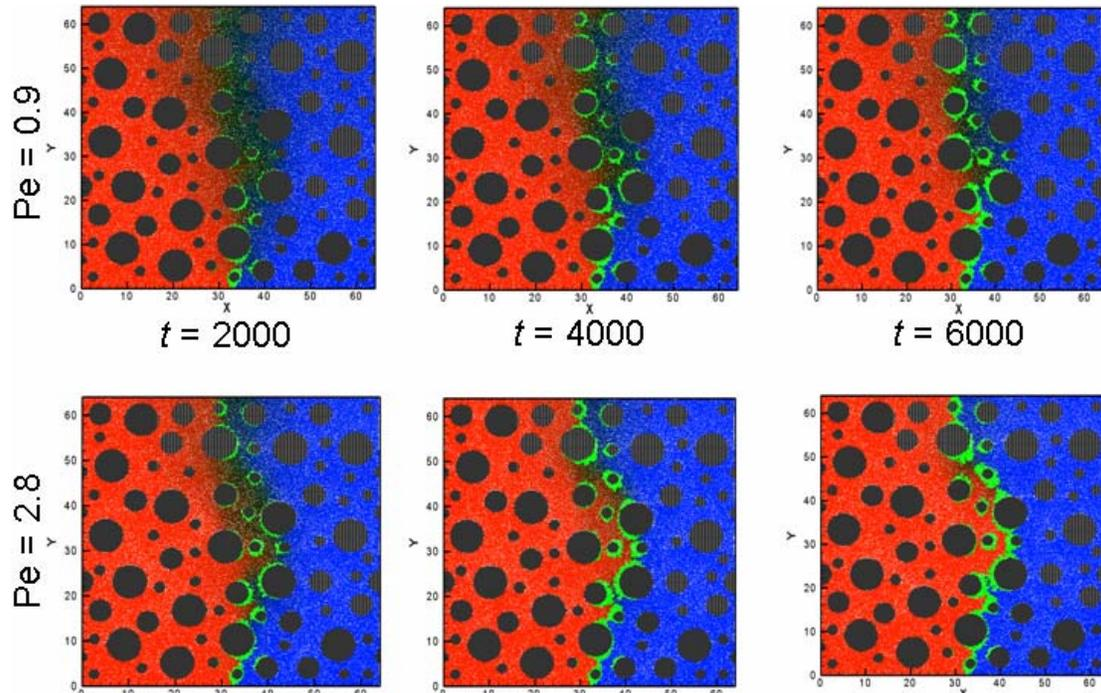
FIGURE 1. Flow and precipitation for two Peclet numbers.
