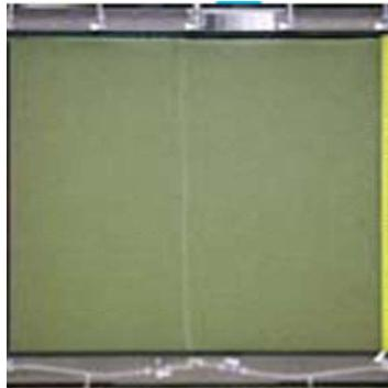
FIGURE 2.  $\text{Na}_2\text{CO}_3$  and  $\text{CaCl}_2$  solutions injected separately at the bottom of the different halves of a vertical 60cm x 60 cm flow cell. The white line in the middle of flow cell is a zone of calcium carbonate precipitation.
