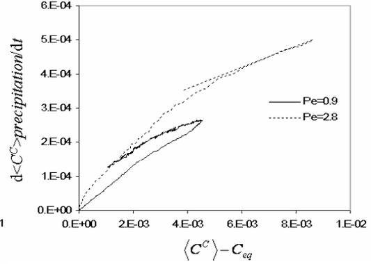
FIGURE 4. Rate of change of  $\langle C^C \rangle$  due to precipitation as a function of  $\langle C^C \rangle - C_{eq}$  for two Peclet numbers.
