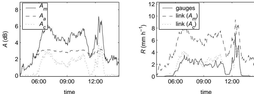
FIGURE 2. Attenuation and rainfall intensity measured the link, compared to the rainfall measured by the gauges. Also shown is the wet antenna attenuation ( $A_a$ ) and its correction ( $A_c$ ), on June 5, 1999.
