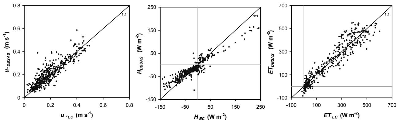
FIGURE 1. Displaced-Beam Small Aperture Scintillometer (DBSAS) fluxes versus Eddy-Covariance (EC) flux estimates during RAPID.  $u_*$  is friction velocity,  $H$  sensible heat flux and  $ET$  Evapotranspiration.
